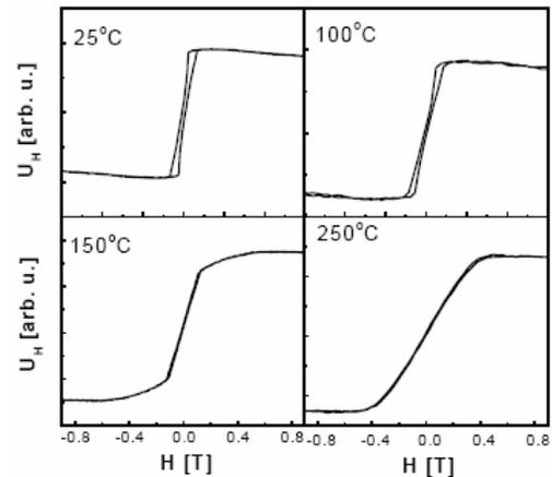
Fig. 4. Hall voltage loops  $U_H(H)$  for MIs deposited at temperatures 100°C, 150°C and 250°C. The  $U_H(H)$  for MI deposited at room temperature is set as a reference.
