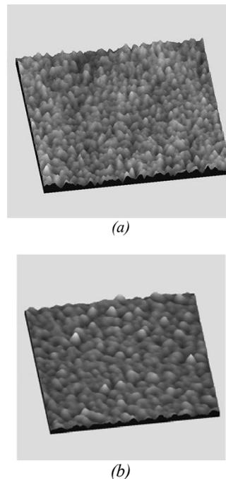
Fig. 2. The STM images ( $1\mu\text{m}^2$ ) of the multilayers  $[\text{Py}(2\text{nm})/\text{Au}(2\text{nm})/\text{Co}(0.8\text{nm})/\text{Au}(2\text{nm})]_{15}$  deposited at  $100^\circ\text{C}$  (a) and  $200^\circ\text{C}$  (b) with the RMS of  $0.27\text{nm}$  and  $0.43\text{nm}$ , respectively.
