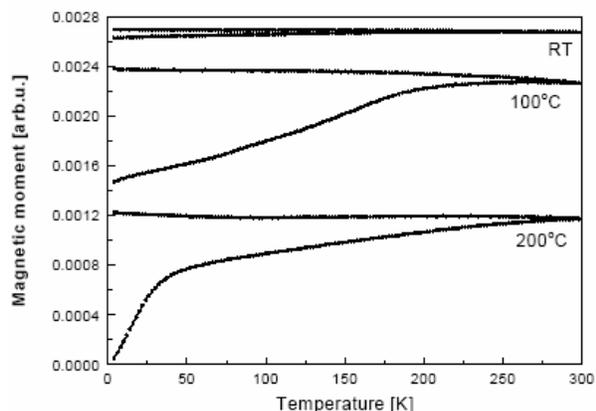
Fig. 6. The normalized FC-ZFC for Mls deposited in different temperatures. Only for the Ml deposited at room temperature the superparamagnetic contribution is not observed. Second two exemplary FC-ZFC curves evidence the presence of the superparamagnetic phase in Mls deposited at 100°C and 200°C.
