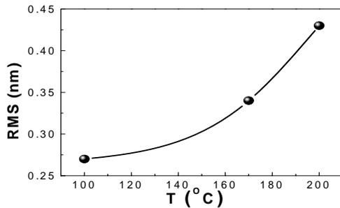
Fig. 3. The RMS values for MIs deposited in different temperatures, measured with the STM.
