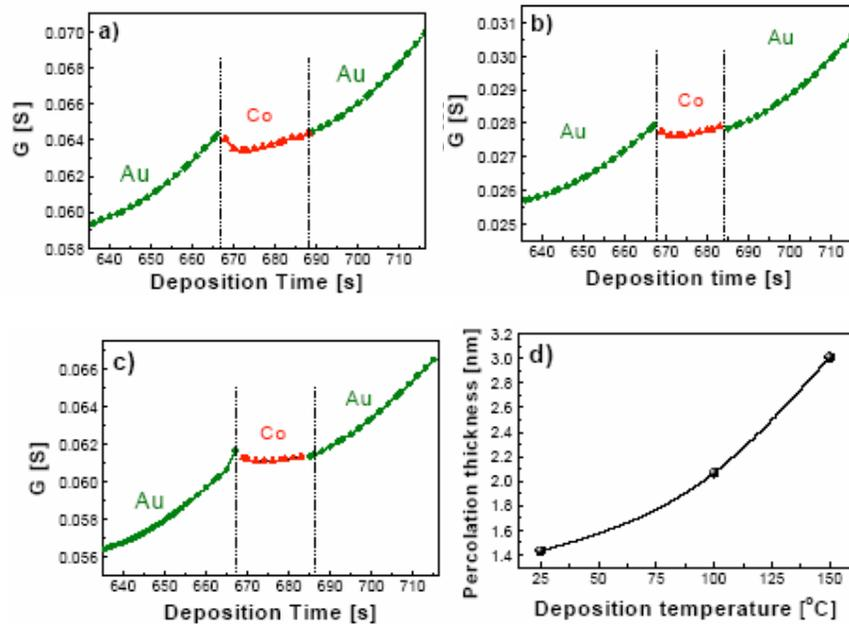
Fig. 5. The  $G(t)$  dependences for Co layer and adjacent Au layers for MIs deposited at a) RT, b) 100°C, and c) 150°C. d) the percolation threshold for MIs deposited at different temperatures.
