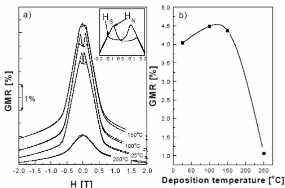
Fig. 1. (a) The GMR(H) for MIs of the composition  $[\text{Py}(2\text{nm})/\text{Au}(2\text{nm})/\text{Co}(0.8\text{nm})/\text{Au}(2\text{nm})]_{15}$  deposited at room temperature, at  $100^\circ\text{C}$ ,  $150^\circ\text{C}$  and  $250^\circ\text{C}$ . The nucleation field  $H_N$  and the annihilation field  $H_S$  are defined in the inset at an exemplary curve. (b) The GMR dependence on the deposition temperature.
