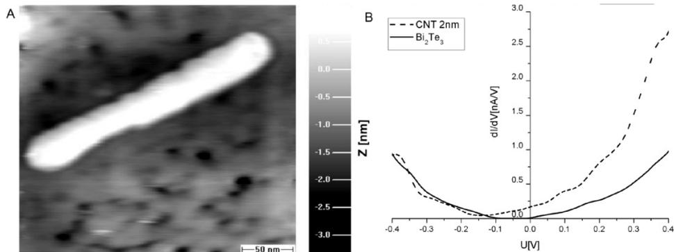
**Figure 4.** (A) STM image of a double-walled CNT2nm about 250 nm long. (B)  $dI/dV$  curves taken over the CNT and the  $\text{Bi}_2\text{Te}_3$  substrate.
