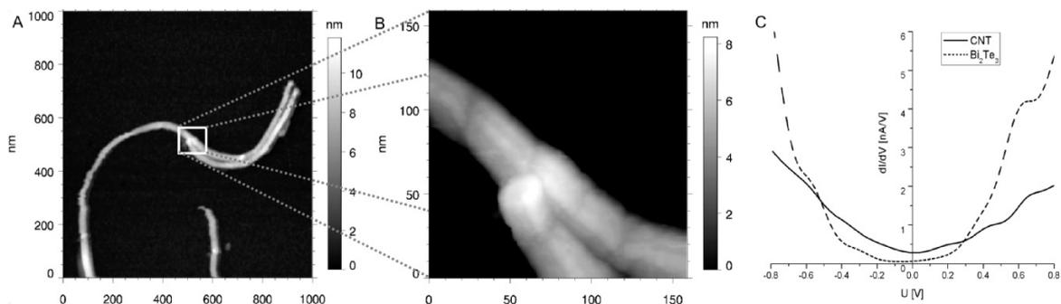
**Figure 2.** (A) STM image of a CNT with a Y junction; (B) higher magnification of the junction area with visible scales along the nanotube; (C) averaged  $dI/dV$  curves taken over the CNT and the  $\text{Bi}_2\text{Te}_3$  substrate.
