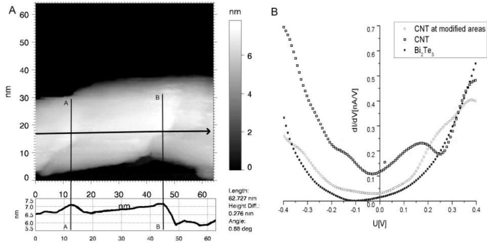
**Figure 3.** (A) STM topography image of a CNT with profile line below. Lines A and B indicate junctions between CNT sections. The image range is  $65 \times 65 \text{ nm}^2$ . (B) Superimposed plot of  $dI/dV$  curves taken over a CNT thickening, along the CNT, and over the substrate.
