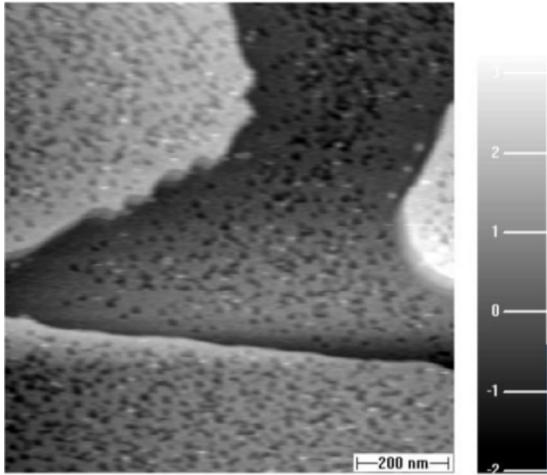
**Figure 1.** STM image of the  $\text{Bi}_2\text{Te}_3$  surface etched by heating at 420 K for a few hours (scan range  $1 \times 1 \mu\text{m}^2$ ). The step height and the hole depth are 1 nm, approximately.
