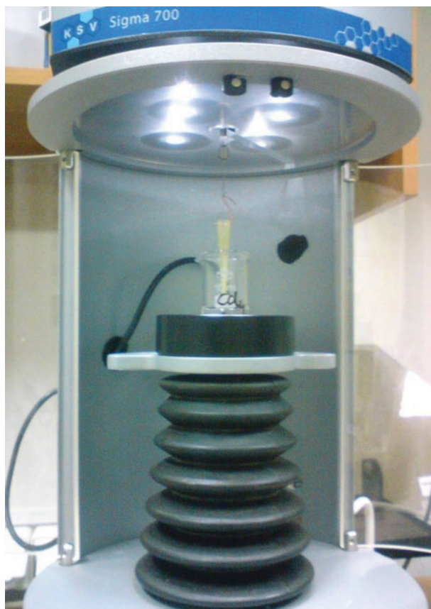
Figure 3. The tensiometer used to study porous solids.
